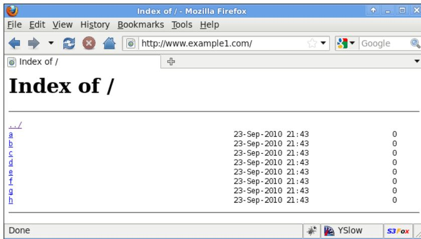
This image displays a sample index auto-generated by Nginx using the preceding configuration. You can see the filenames, timestamp, and the file sizes as the three data columns.
